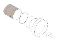
Inlet connection with  $\emptyset$  dimensions different from the inlet bag.
