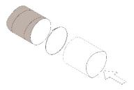
Inlet connection with the same  $\emptyset$  dimensions as the inlet bag.
